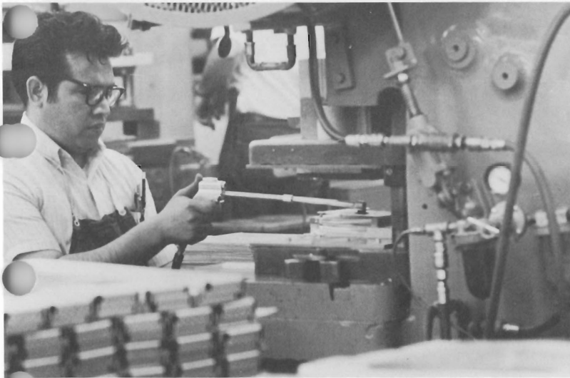
Amador Gonzalez, using a suction cup for safety, puts aluminum front panels into a blanking machine, which punches out meter windows, notches and other cut-out sections. Other machines perforate, punch and form the raw sheet before it's ready for painting, engraving and final assembly.
