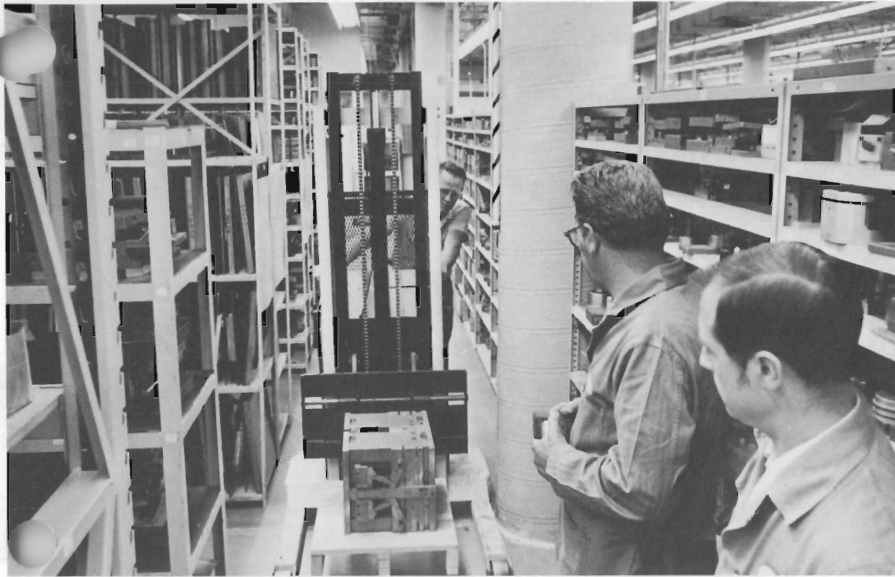
Close to $3 million is invested in steel rule dies, die sets, BL units and stamps "librared" in Manufacturing Division's tool crib. Each of the dies and sets is used to make a single part from aluminum sheet for a certain instrument, and it's estimated that each of the nearly 4,000 dies, sets and molds gets used at least once every nine months. Here, Buddy Franklin, Aldo Paganinni and Don Knox "check out" a die set.
